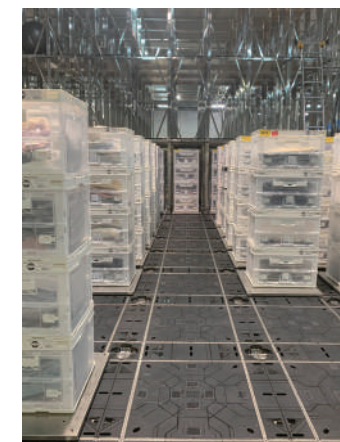
Self-propelled magnetic trays run on linear motor tiles
